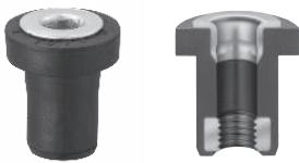
● Allows the fastening screw to be tightened without torque control because of the metal sleeve attached in the WELL Nut.
